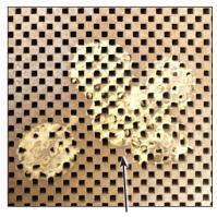
Broken or Cracked Ceramic
